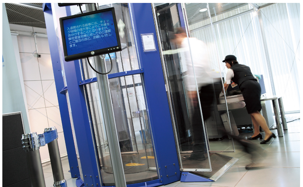
A 3D holographic scanner installed at a data center entry/exit point
